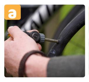
Use your pump to inflate the tube and check for the hole (a).
