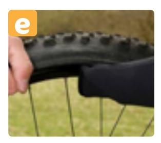
From here either mend the puncture (see the Mending Punctures section), or get a new inner tube out ready to fit.
