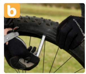
Use a second tyre lever if necessary in exactly the same way. Insert it under the bead 50 - 75mm (2 – 3") away from the first (c). The tyre should now be loose enough for the tyre bead to be pulled off the rim all the way round. Note that only one side of the tyre is removed; the other bead remains on the rim.
