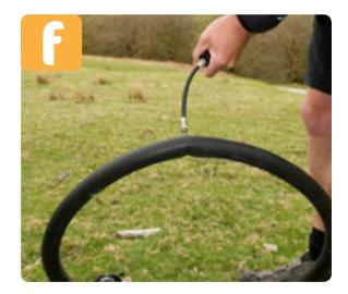
Insert the valve into the valve hole in the rim and push the tube inside the tyre and into the rim. The tyre bead can then be replaced under the rim edge (g). Avoid leaving the valve area until last as this often pinches the tube. The valve may just need pushing into the rim slightly to help the tyre seat properly at this point.
