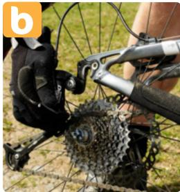
Line the rear wheel up with disc brake calliper (if fitted) and drop outs and push it into position (c).
