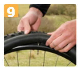
Inflate the tube until it fills the tyre and reaches a soft squashy pressure. At this point go around the tyre flexing it over the rim on each side. This helps seat the tyre squarely on the rim all the way round.
