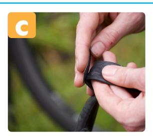
Peel the backing from self-adhesive patch and press patch firmly onto the tube. The tube must be clean and dry for the patch to adhere properly.
