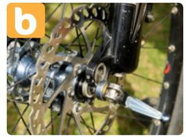
Adjust the quick release nut appropriately and tighten the quick release into place.
