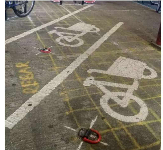
Examples of ground anchors and reserved spaces for non-standard cycles
